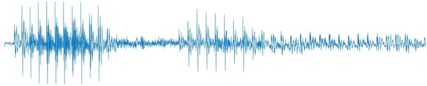
Fig. 2. The time characteristics for the word "seven"
